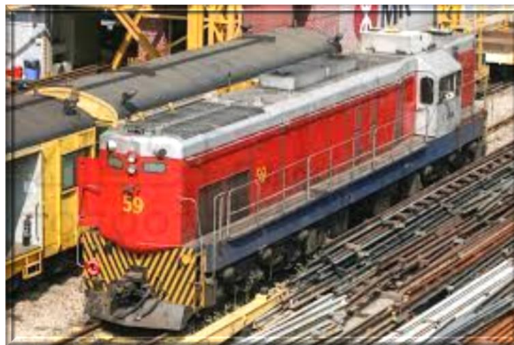
G. M. Model G16 Diesel Electric Locomotive No.59 was named "Gerry Forsgate" (霍士傑號) in commemorating the first Chairman of the Kowloon-Canton Railway Corporation.
