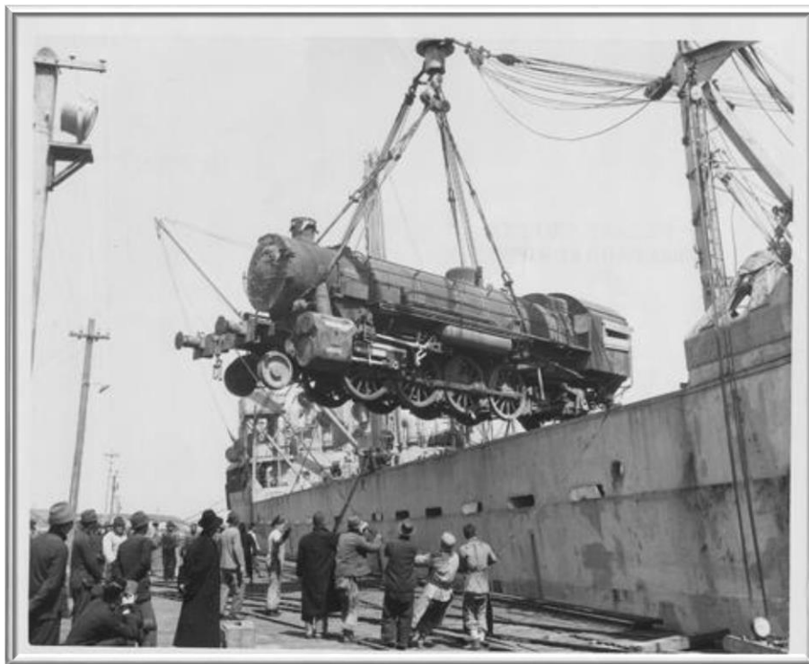
1946年 -- 上海吳淞碼頭工人卸下聯合國善後救濟總署提供的機車頭。 A fully-assembled, 90-ton "MacArthur" type railroad locomotive being unloaded at Shanghai's Woosung docks to be used in UNRRA's rehabilitation of China's railroad. (1946)
